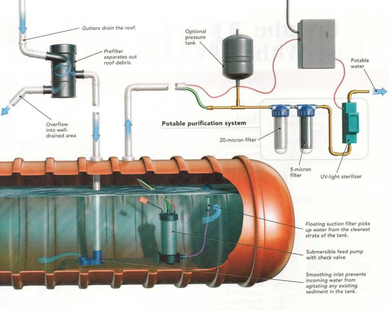
of four. A potable collection system is identical to a nonpotable system except that it intercepts the indoor-bound water with a series of filters. The typical setup consists of a three-stage filtration process in which water is pumped successively through a 20-micron charcoal filter and a 5-micron filter and then is sterilized by an ultraviolet light. This array of filters only adds \$1500 to \$2000 to the overall cost of a system.
