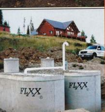
Concrete. Typically used for larger storage (1000 gal. or more), concrete cisterns are formed and poured below grade. The tops are formed and poured on site, then lifted into place. Concrete cisterns cost about \$1.25 per gal.
