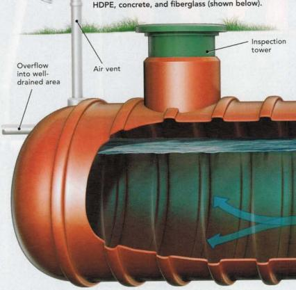
ing bacterial growth. Choices include corrugated-steel or aluminum shells that bolt together around a heavy-duty plastic liner, high-density polyethylene (HDPE), and fiberglass. There's also a unit called the Rainwater Pillow (rainwaterpillow.com), essentially a composite bladder that can hold up to 20,000 gal., that's designed to be stored in a crawlspace or under a porch.
